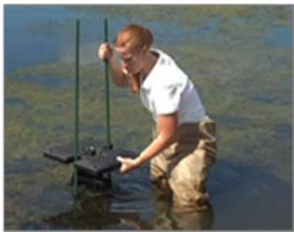
SonicSolutions® device installation using stakes.
