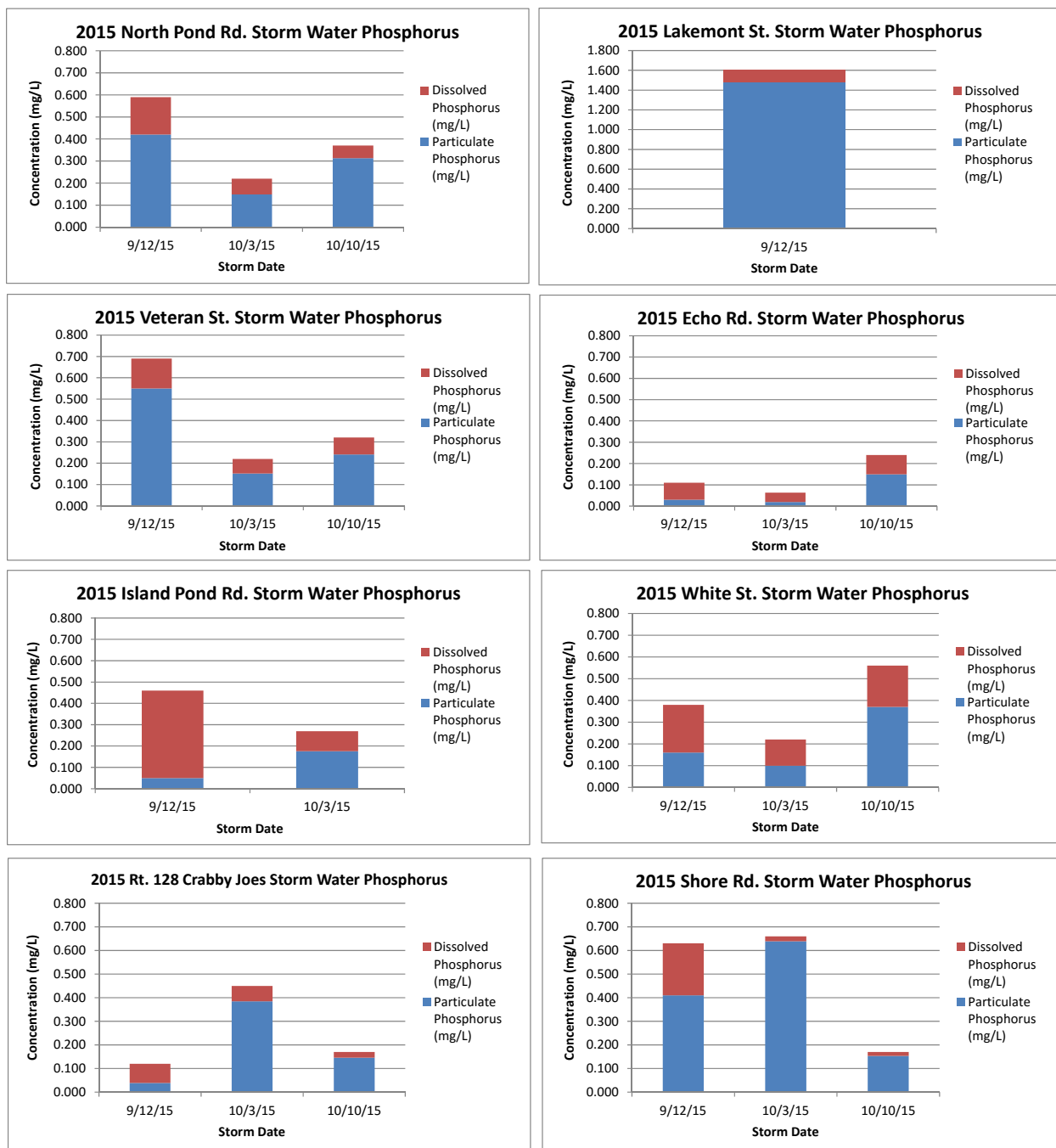
Figure 23. Storm Water Phosphorus in the Congamond Lakes Watershed in 2015
