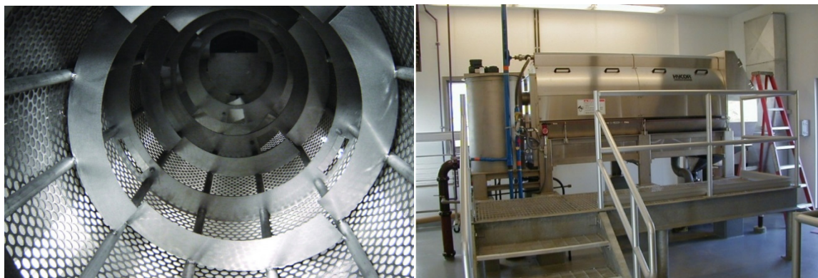
Figure 6: Example of Rotary Drum Thickener (Parkson Corporation)
