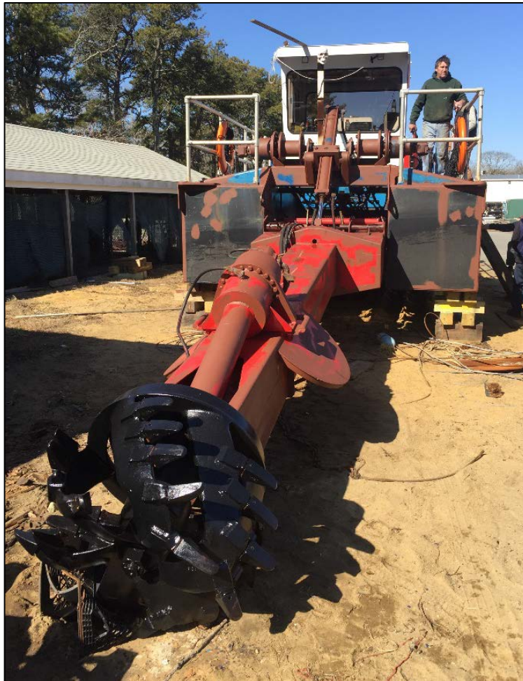
Figure 17. The cutter head of the Town of Edgartown Ellicott-370 hydraulic dredge, in the municipal lot for annual maintenance.
