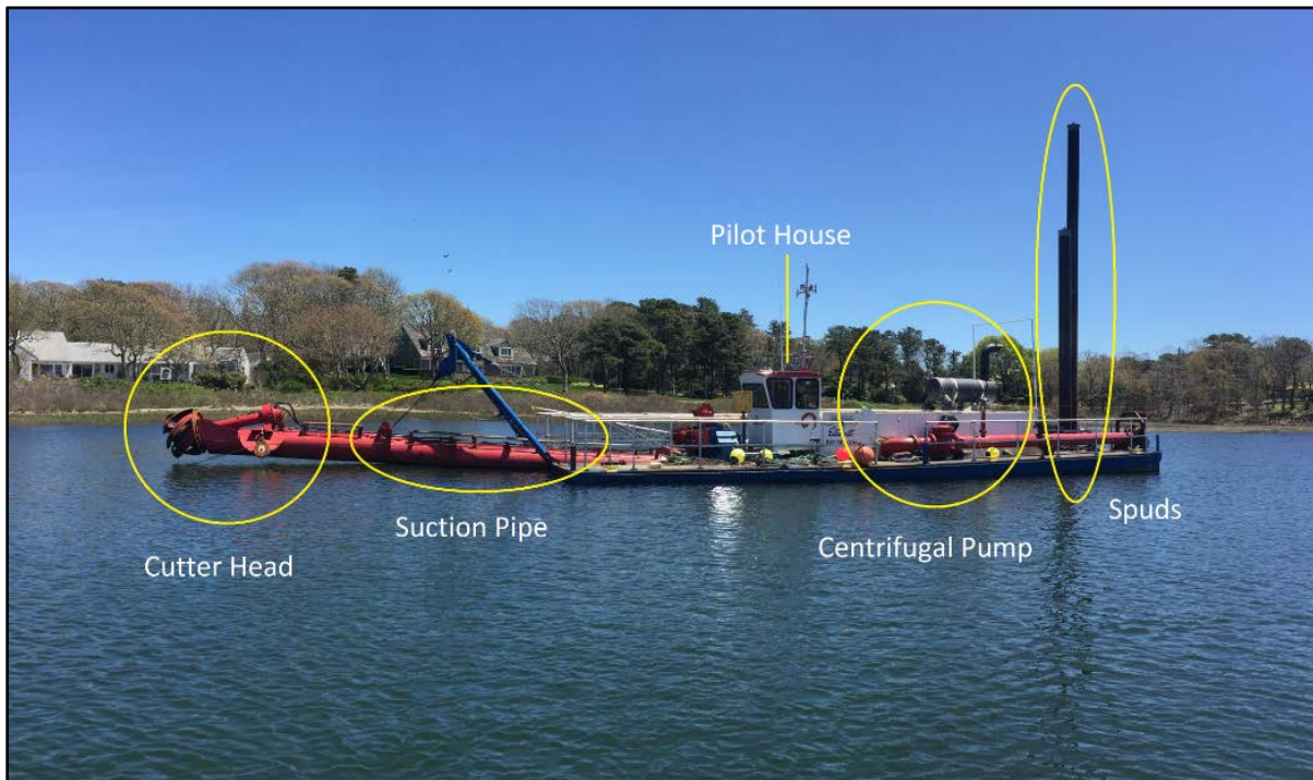
Figure 3. Components of a Barnstable County Dredge Superstructure, a Hydraulic Cutter Suction Dredge at rest in Saquatucket Harbor, Harwich, MA, May 2019.
