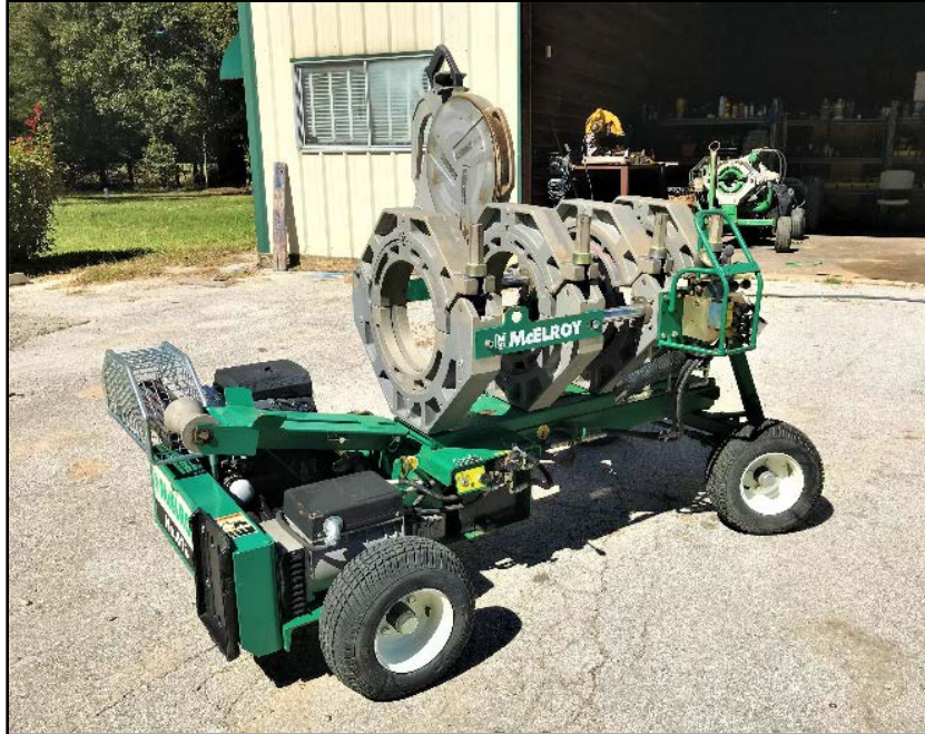
Figure 10. Typical pipe fusion machine. Retrieved 21 July 2020. https://www.westerndredge.com/product/mcelroy-618-fusing-machine/
