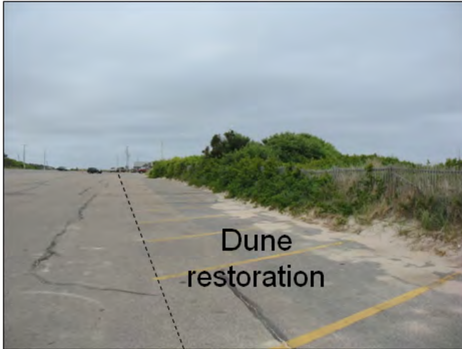
Figure 26. Suggested area of parking lot to be removed to accommodate a dune restoration project during Phase 2 of the Phased Retreat Plan.
