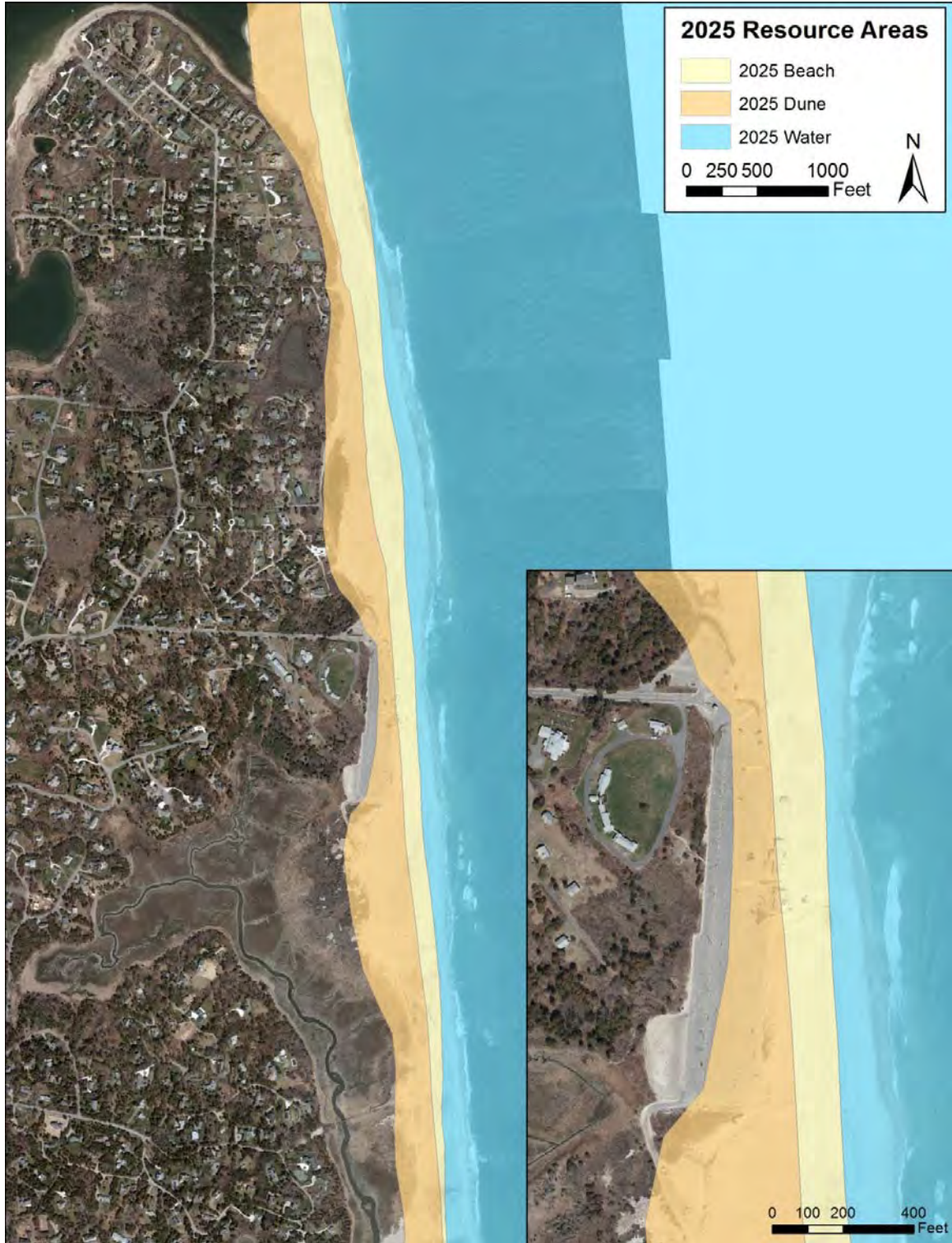
Figure 15. Projected positions of the coastal beach and coastal dune at Nauset Beach after 10 years.
