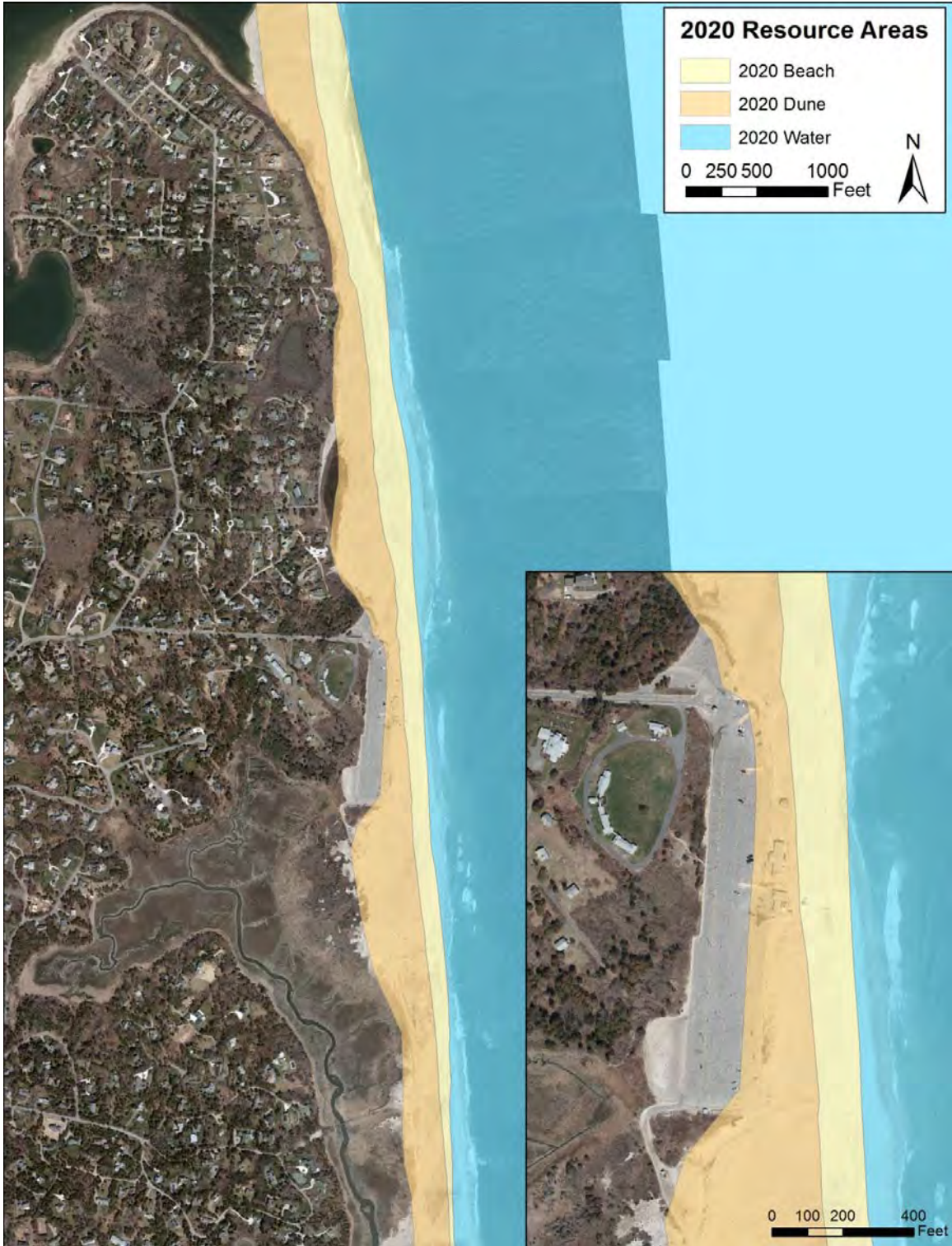
Figure 14. Projected positions of the coastal beach and coastal dune at Nauset Beach after 5 years.
