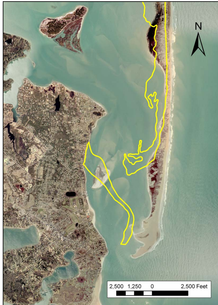
Figure 5. Conceptualization of a single north inlet used for the development of the water quality model run of scenario two.
